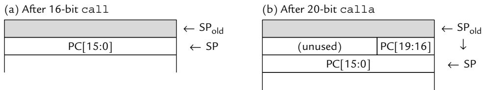
Figure 11.3: Stack after calling a subroutine with (a) call in the MSP430 and (b) calla in the MSP430X. Two words on the stack are needed to store the 20-bit return address after calla .
