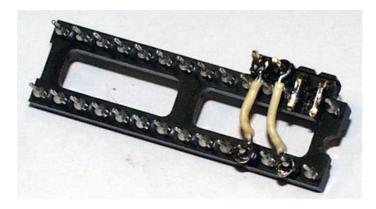
Make sure that the two wires attached to pins 2 (Vdd) and 4 (Vss) of the upper socket are located as close as possible to the plastic part of the socket without touching other socket pins.
