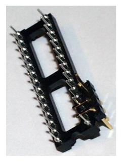
Make sure that the two bent header pins are as close as possible to the two matching socket pins (pin 27 - OSC1 and pin 26 - OSC2).
