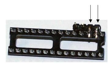
Next, we need to connect the remaining two straight header pins to the Vdd (pin 2) and Vcc (pin 4) upper socket pins. Use two short pieces of the isolated wires to make your "masterpiece" look like this:
