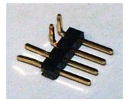
If you are using an "all-straight" header, bend the upper two pins by 90°. If you have a 90° header, bend the lower two pins straight.
