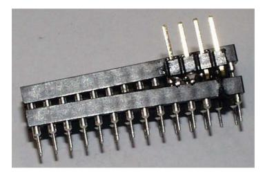
Although this assembly looks a bit "beveled", it will work fine, as long as all pins of the upper socket (except pin 27 – OSC1) contact the lower socket's pins.
