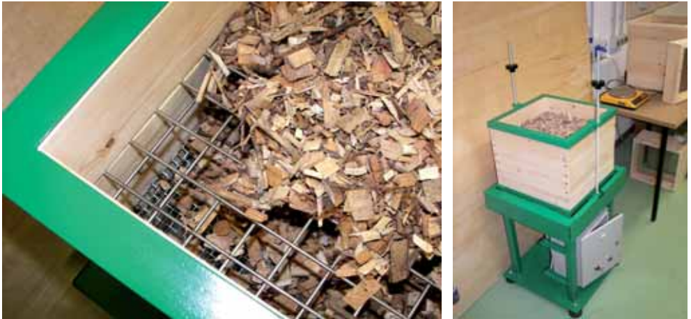
Figure 4.3.1 Device for wood chips size determination (AIEL 2006)
