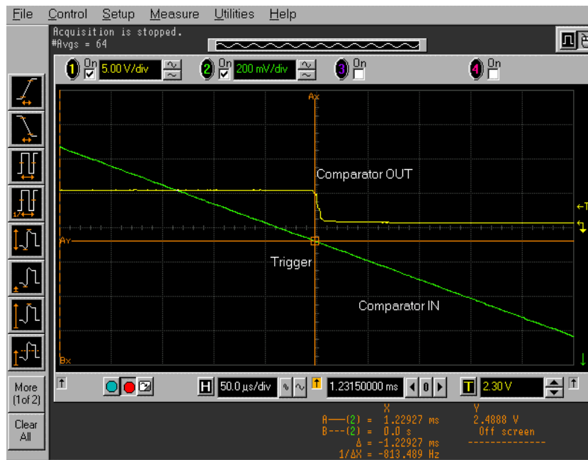
Figure 3-2. Transfer Characteristic of Digital CMOS Input with Linearly Decreasing Input Voltage
