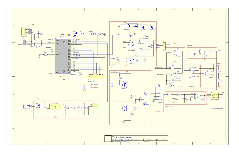
This schematic shows the latest revision of the hardware. It includes hardware for output since it is used for the half-duplex modem application, which is unnecessary for the Caller-ID application. Keep in touch with <u>www.scenix.com</u> for any updates we make available.
