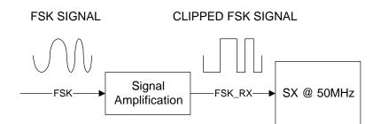
The software implementation of FSK detection is very simple. The transitions on the input pin are timed by the software. If the transitions occur within a specified time, then a high frequency is being detected, otherwise a low frequency is being detected.
