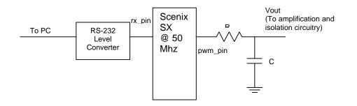
Depending on the maximum frequency you wish to obtain, you should adjust the component values for R and C to choose the resolution of the PWM. Ideally, you should calculate the maximum SIN frequency output you will use and choose the cutoff to be at this frequency. For instance, for a maximum output frequency of 2.1kHz, calculate R and C:
