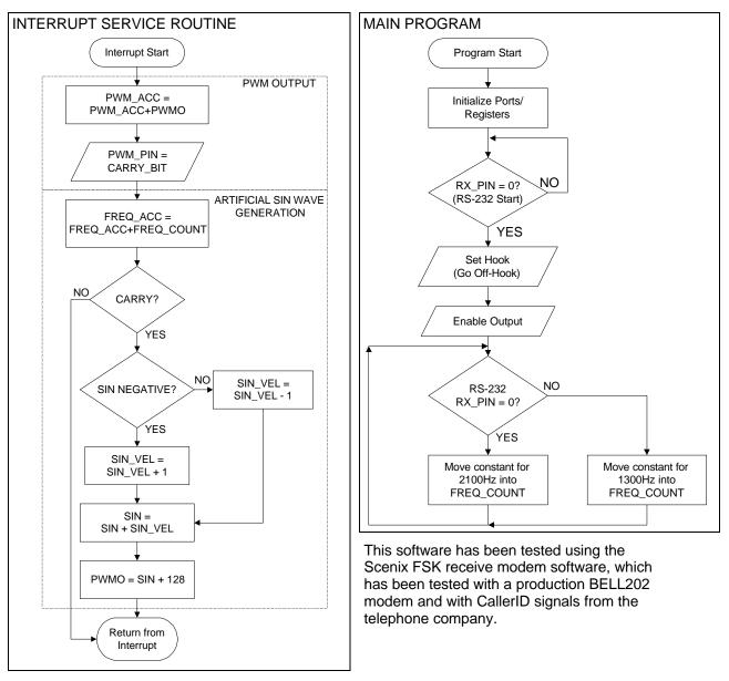
This is an extremely simple method to perform FSK modulation. To make the system more powerful, an RS-232 UART could be added so the incoming RS-232 data can be processed (Required to implement an AT-command set). To create a full modem solution, this software module must be combined with the FSK receive module and the DTMF transmit (Dialing) module.
